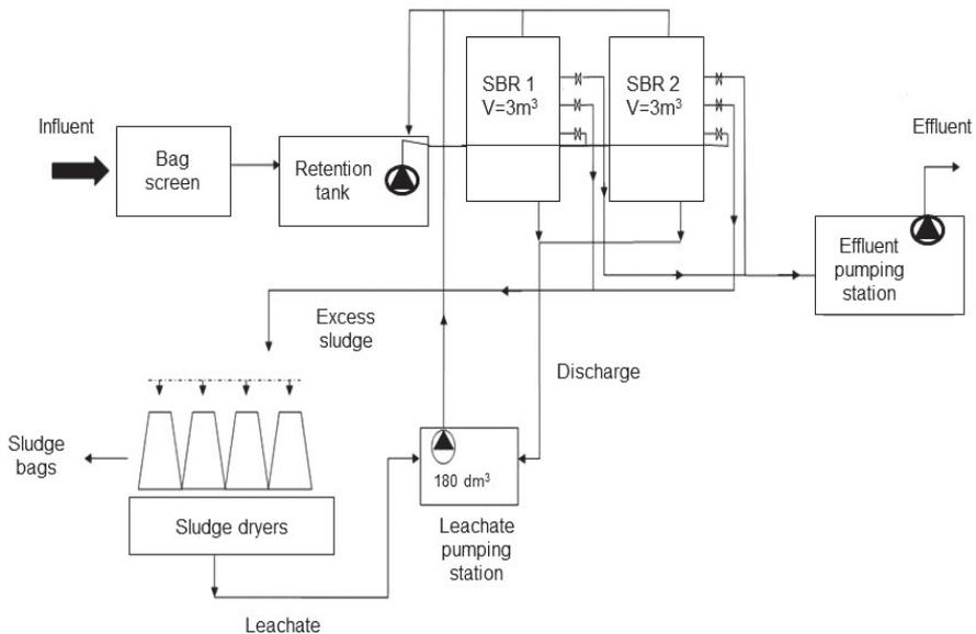
Fig. 4. Flow chart of the West Spitsbergen wastewater treatment plant [10]
