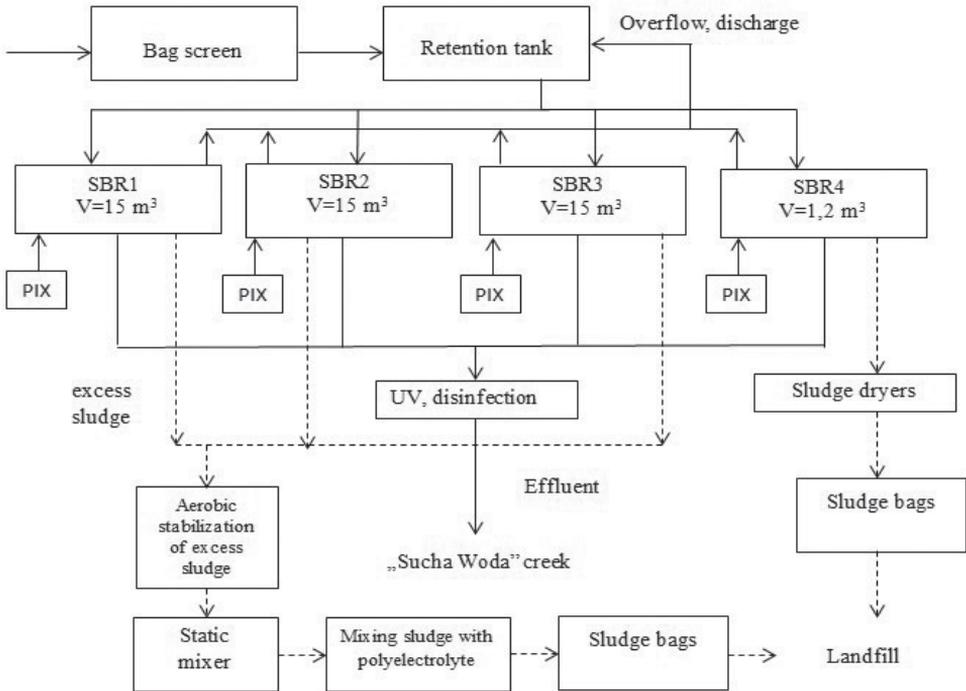
Fig. 5. Flow chart of the Murowaniec wastewater treatment plant [10]
