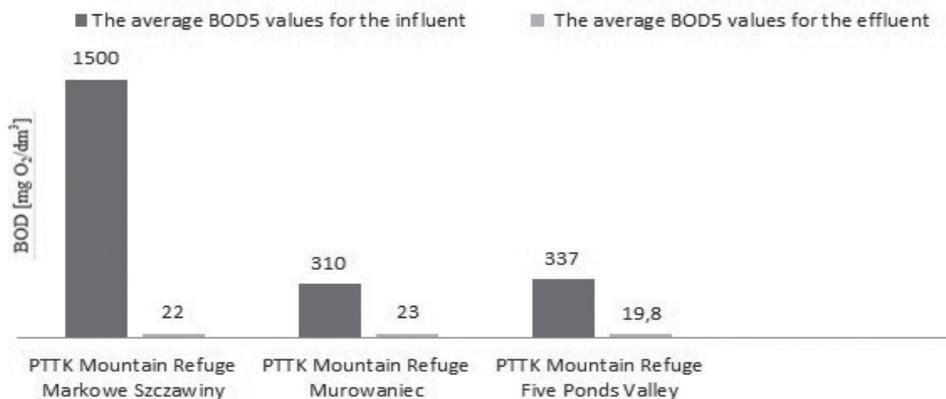
Fig. 9. BOD<sub>5</sub> in the raw sewage and in the effluent from the mountain hostels
