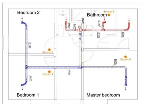
Fig. 3. First floor – sensor layout
