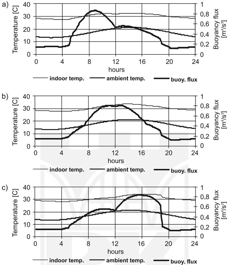
Fig. 1. Time history of indoor and outdoor temperature and buoyancy flux in July in Warsaw without influence of wind, wwr equals 50%, insulation layer equals 30 cm: a) east, b) south, c) west window
