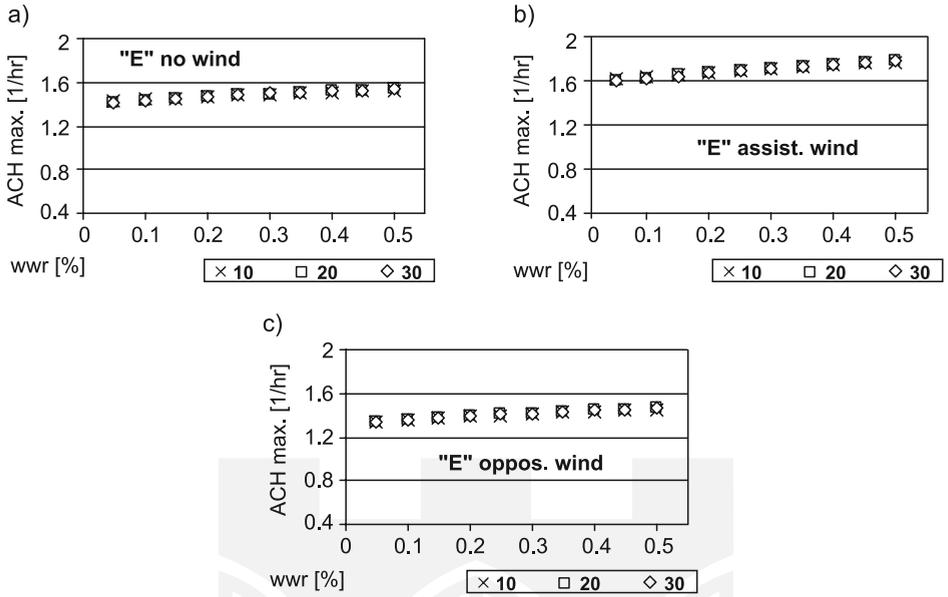
Fig. 4. Max. ACH at the east window in July in Warsaw: a) no wind, b) assisting, c) opposing wind
