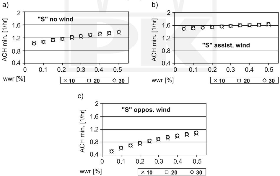
Fig. 5. Min. ACH at the south window in July in Warsaw: a) no wind, b) assisting, c) opposing wind
