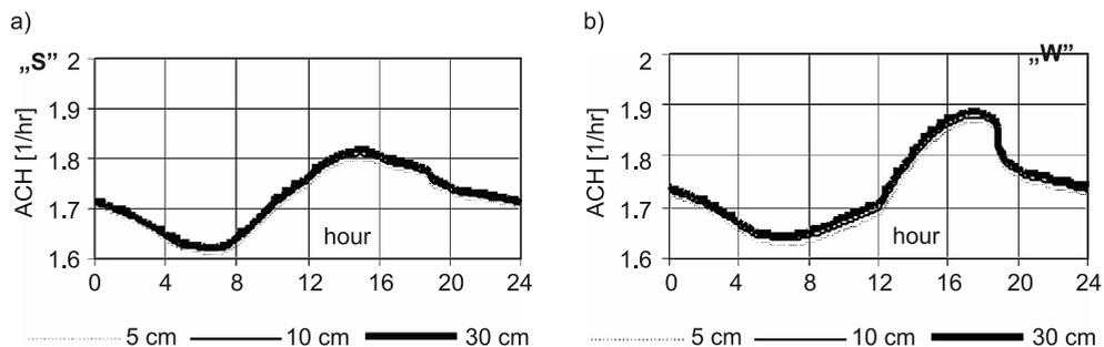
Fig. 2. Time history of air rate change rate at different insulation in July in Warsaw when wind appearances are not observed (without influence of wind), window surface to wall area (wwr) equals 50%: a) south orientation; b) west orientation
