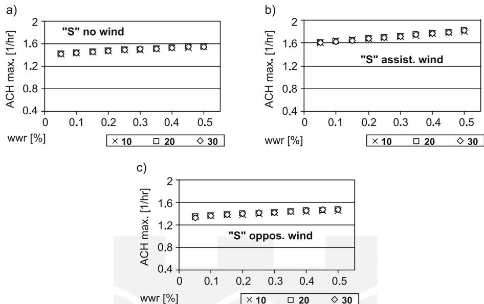
Fig. 6. Max. ACH at the south window in July in Warsaw: a) no wind, b) assisting, c) opposing wind
