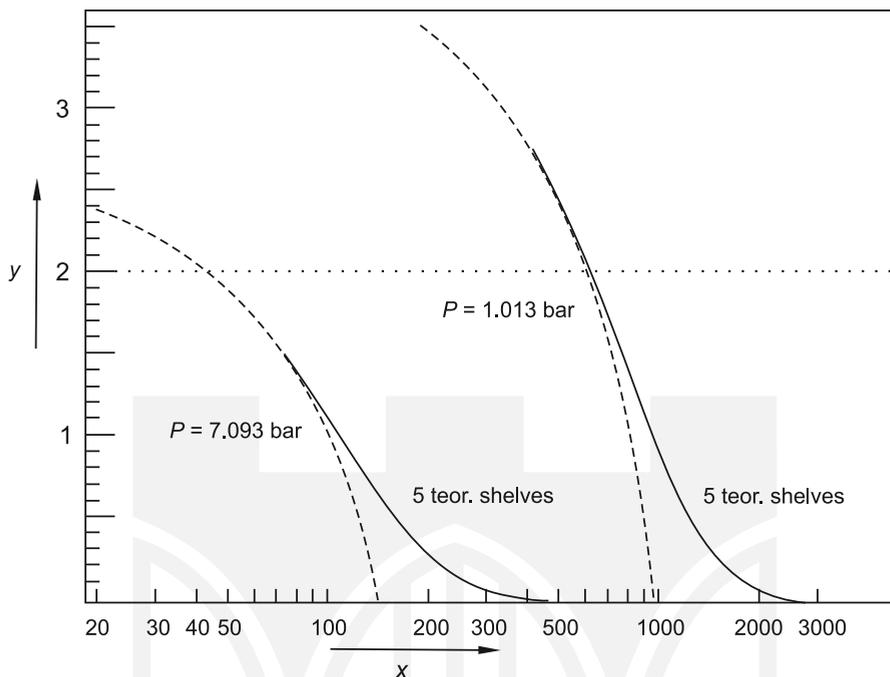
Fig. 8. Comparison of nitric oxide concentration in gas leaving the absorption stage under atmospheric pressure and under higher pressures. Common conditions:  $T = 303 \text{ K}$ ;  $A_1 = 2$ ;  $B_1 = 0$ ;  $S_1 = 0$ ;  $M = 30\%$ . The absorption system is adequate for five theoretical shelves (continuous lines), broken lines correspond to an unlimited number of theoretical shelves. The right pair of curves relates to the atmospheric pressure, the left pair relates to a pressure of 7.093 bars
