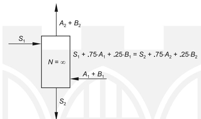
Fig. 4. Scheme of an absorption system with an unlimited number of theoretical shelves.
