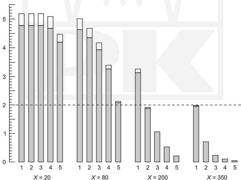
Fig. 10. Nitrogen oxide content after each shelf in an absorption system adequate to five theoretical shelves. Initial conditions:  $T = 303$  K;  $P = 7.093$  bars;  $M = 55\%$ ;  $A_1 = 2$  (0.2% vol.);  $B_1 = 0$ ,  $S_1 = 0$ . For further explanation, see Fig. 9
