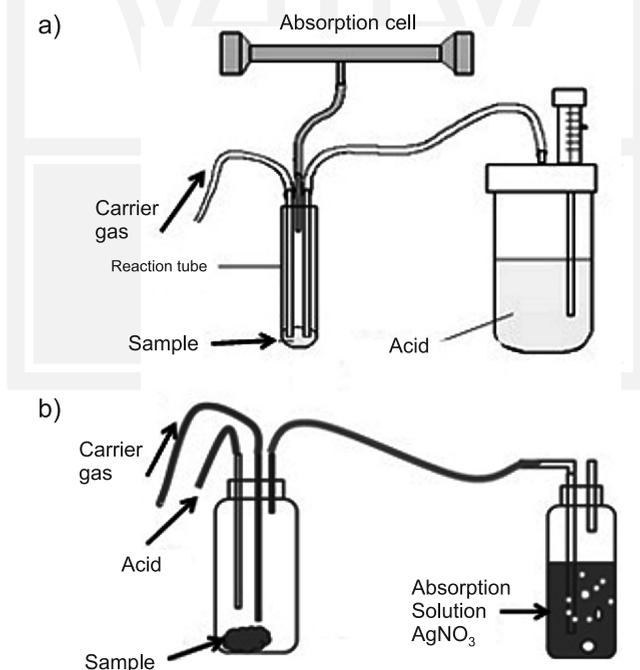
Fig. 1. The measurement systems: a) the system where the  $\text{H}_2\text{S}$  is measured by molecular absorption and b) the system where the liberated  $\text{H}_2\text{S}$  is absorbed and precipitated
