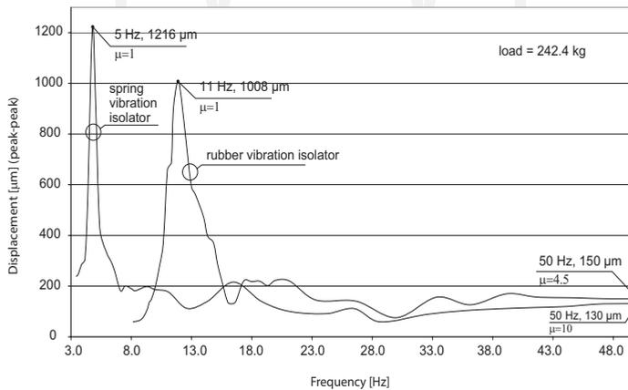
Fig. 4. Displacement (peak-peak) of vibration platform based on a rubber and spring in a function of driving frequency
