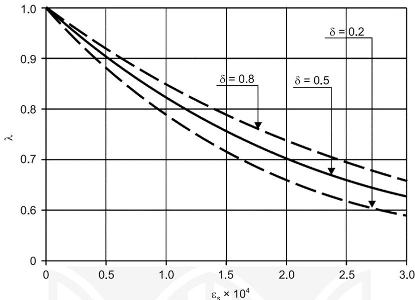
Fig. 4. Effect of concrete free shrinkage  $\epsilon_s$  and rigidity of steel girder and connected reinforced concrete slab ( $\delta$ ) on coefficient  $\lambda$ .
