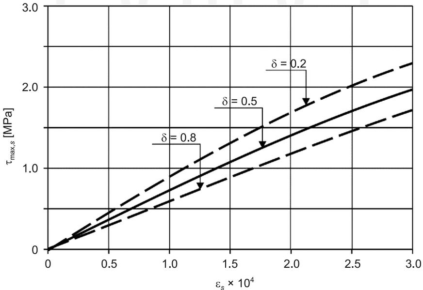
Fig. 3. Effect of concrete free shrinkage  $\varepsilon_s$  and rigidity of steel girder and connected reinforced concrete slab ( $\delta$ ) on shrinkage stresses  $\tau$  in connection plane
