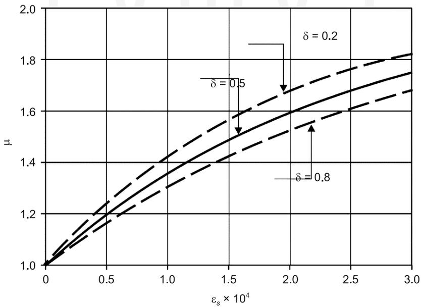
Fig. 6. Effect of concrete free shrinkage  $\epsilon_s$  and rigidity of steel girder and connected reinforced concrete slab ( $\delta$ ) on coefficient  $\mu$  at  $\kappa = 0.5\mu$  and at  $\kappa = 0.7$
