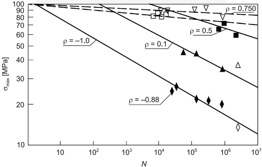
Fig. 1. Results of fatigue tests on flexible connectors [4]
