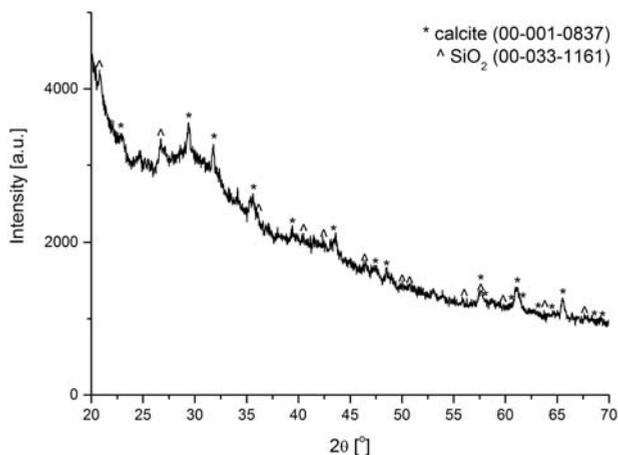
**Fig. 7.** Powder diffraction pattern of the green paint layer for the sample taken from the painting *Model of the World*
