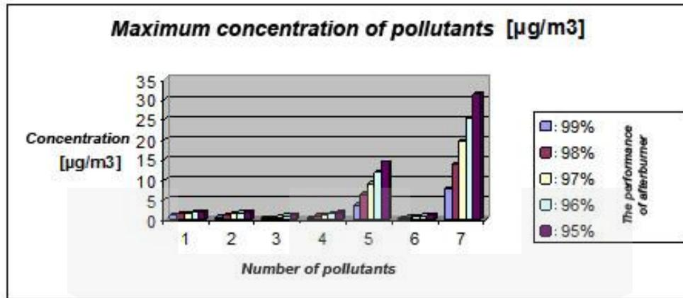
Fig. 3. A graph showing maximum concentration of selected impurities depending on the performance of afterburner
