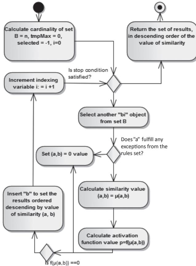
Fig. 1. UML activity diagram of compound object comparator
