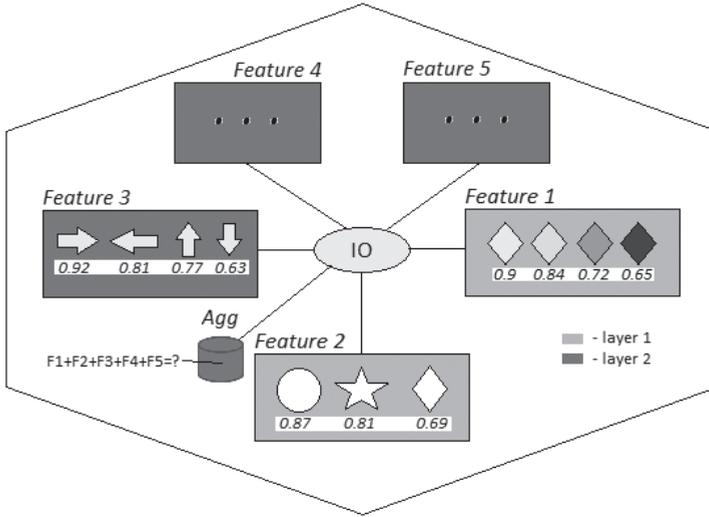
Fig. 3. General schema of signal granule used for transfer of information between comparators, aggregators, layers, in the network of comparators. Feature  $n$  – processed feature, IO – input object, Agg – aggregated data
