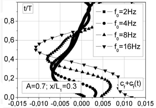
Fig. 4. Time dependent distributions of the wall shear stress coefficient obtained from numerical simulation for inflow amplitude  $A = 0.2$  (a, b) and  $A = 0.7$  (c, d) at upwind  $x/L_1 = -0.3$  (a, c) and downwind  $x/L_1 = 0.3$  (b, d) positions
