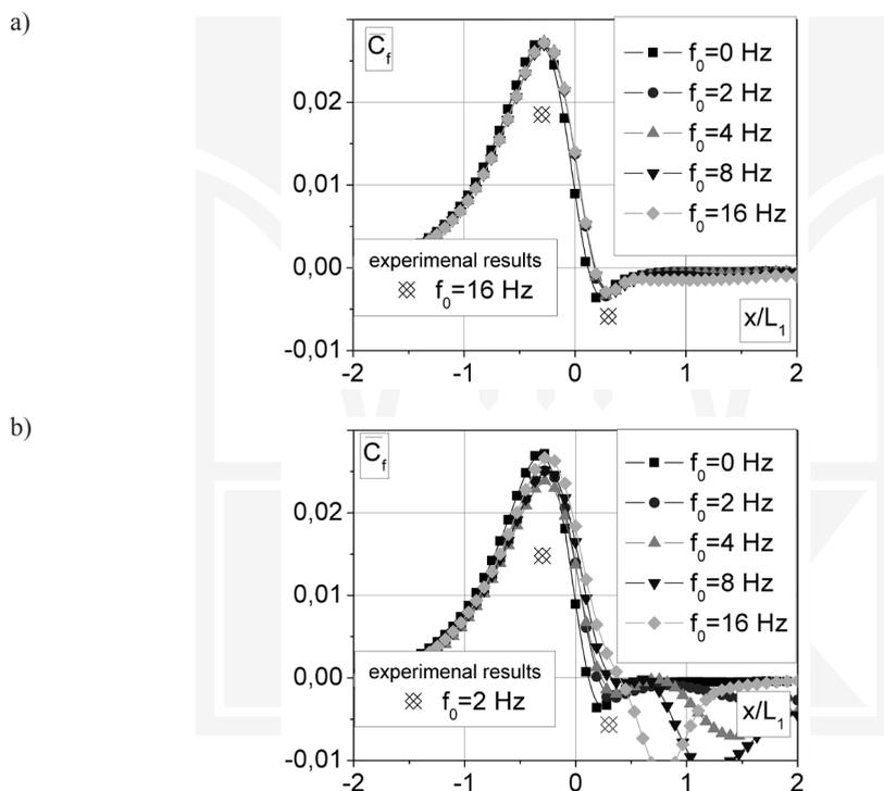
Fig. 3. Distribution of mean wall shear stress coefficient around the hill surface for a) low ( $A = 0.2$ ) and b) high ( $A = 0.7$ ) amplitude of inflow oscillations
