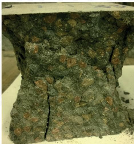
Fig. 4. Typical failure modes of SCC1
