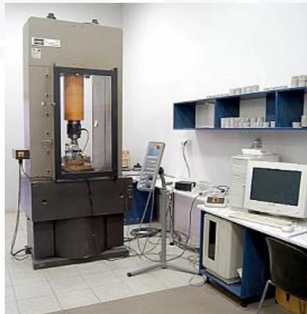
Fig. 2. MTS testing system for uniaxial compression tests
